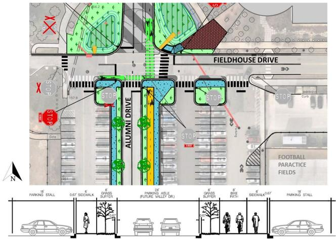
FIGURE 11: PROPOSED PLAN VIEW AND CROSS-SECTION VIEW OF ALUMNI DRIVE THROUGH LOT 1/Z,
