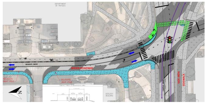
FIGURE 31: PROPOSED REGENTS DRIVE CYCLETRACK AND LANE WIDENING NEAR CAMPUS DR
