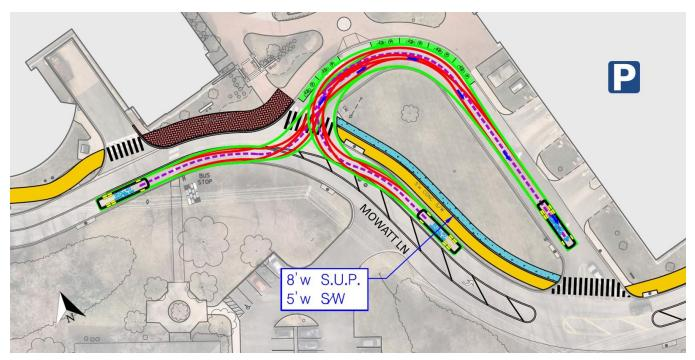
FIGURE 18: PROPOSED SEPARATED BIKING AND WALKING PATHS NEAR MOWATT GARAGE
