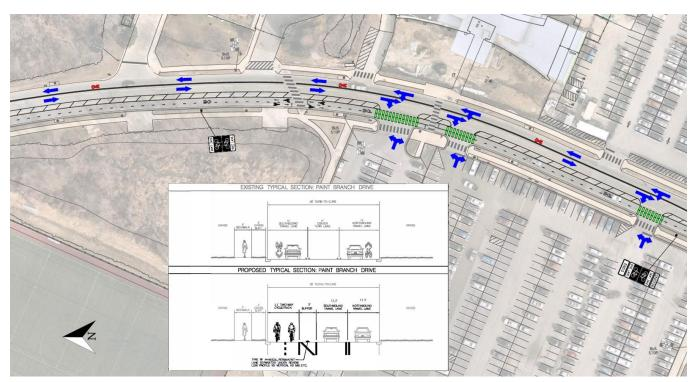
FIGURE 27: PROPOSED PLAN AND CROSS-SECTION FOR INTERIM 2-WAY CYCLETRACK ON PAINT BRANCH DRIVE
