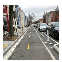
FIGURE 4: VARIOUS ON-ROAD CYCLETRACK VERTICAL PROTECTION ELEMENTS
