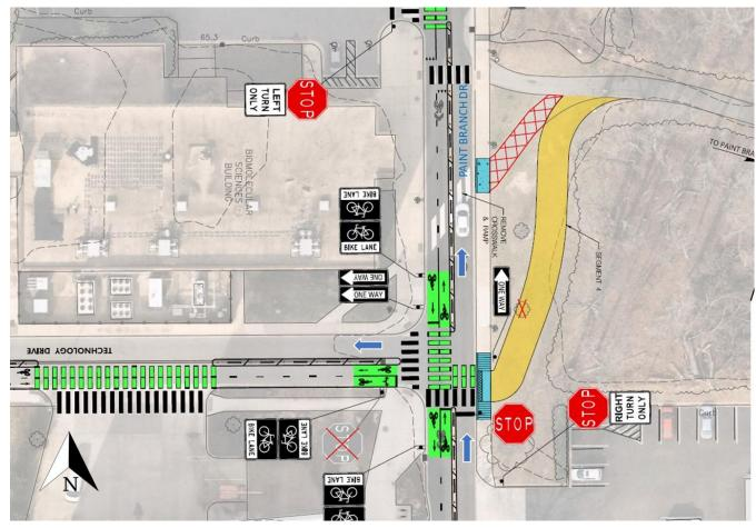
FIGURE 38: PROPOSED CONNECTION FROM PAINT BRANCH TRAIL TO TECHNOLOGY DRIVE
